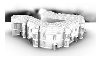
Fig. 26. A procedural model that renders a street from a spline. In this case the street was generated by four points defining the street's curve. Seed points were grown using another application of the skeleton to create the building footprints.
