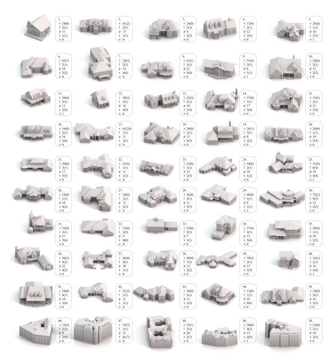
Fig. 25. The example cases and modeling statistics. v Vertices in modeled plan (additional vertices); l Polygons in modeled plan (polygons in library plan); p Number of profile sections in model; s Number of natural steps designed (number of natural step applications); o Number of offset events.
