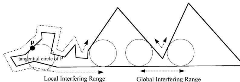
Fig. 6. Interfering point and interfering-range (LIR, GIR).
