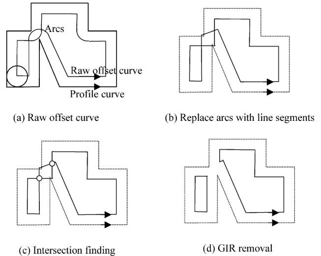
Fig. 7. Procedure of the suggested mitered offsetting algorithm.
