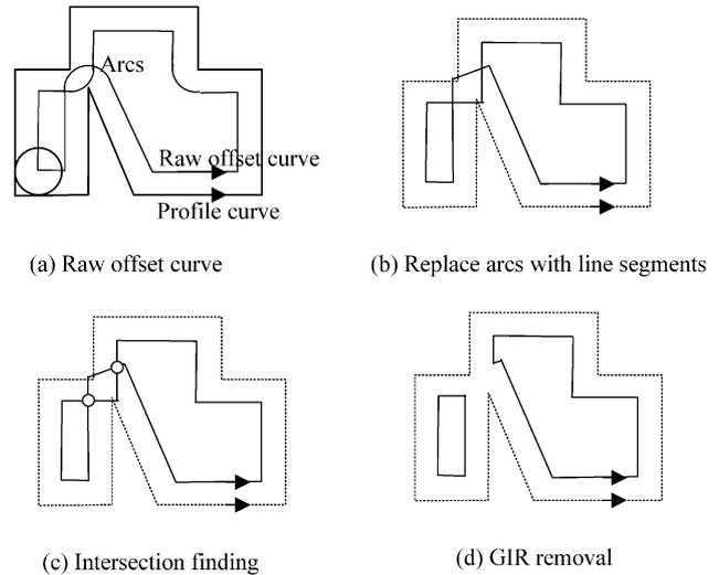
Fig. 7. Procedure of the suggested mitered offsetting algorithm.
