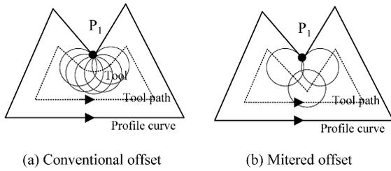
Fig. 1. Conventional offset and mitered offset.
