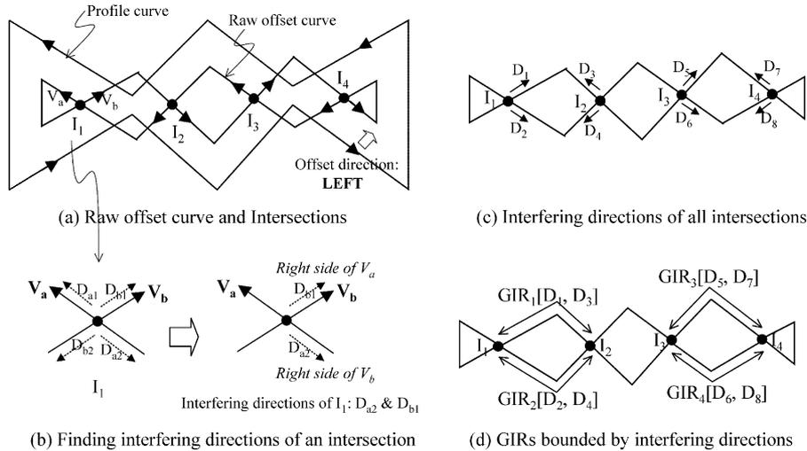
Fig. 8. New GIR removal procedure for mitered offsetting.
