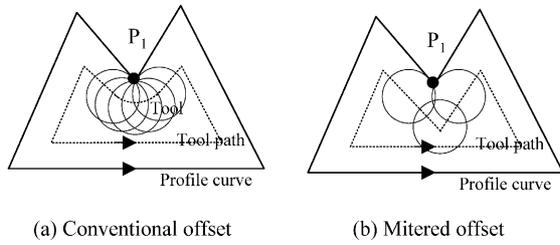
Fig. 1. Conventional offset and mitered offset.
