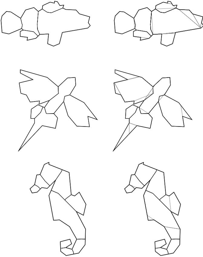
**Figure 11: Examples of the proposed decomposition: the parts resulted after the global splitting (left) are further locally simplified (right), by means of protrusion-cut segments. The boundary of the shape is drawn in thick solid lines, the split-chains in thin solid lines and the protrusions cut segments in dotted lines.**
