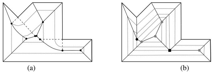
**Figure 1: Medial Axis (a) vs. Straight Line Skeleton (b). In (b) the black disk marks a reflex edge annihilation, while gray disks mark convex edge annihilations. An edge-edge collision generates the arc between the black box (vertex-edge collision) and a gray disk (convex edge annihilation).**
