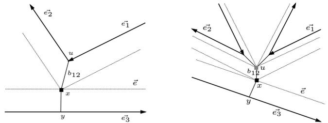
**Figure 7: The reflex vertex generating a vertex-edge collision at  $x$  can originate in a vertex of  $P$  (left) or may have appeared in the propagation process (right). In both cases, the split-chain contains on this side of  $x$  only one segment ( $xu = b_{12}$ ). On the other side of  $x$ , the split-chain contains one segment ( $xy$ ) also, but only when  $y$ , the projection of  $x$  onto the edge that is split, falls inside it.**
