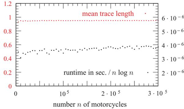
Fig. 5. The runtime of Moca and the mean trace length of random datasets with different numbers  $n$  of motorcycles. The start points are uniformly distributed on  $[0, 1]^2$  and the directions are uniformly distributed on  $[0, 2\pi)$ . For illustrative reasons, we divided the runtime by  $n \log n$  and the mean trace length by  $\sqrt{\frac{\pi}{n-1}}$ .
