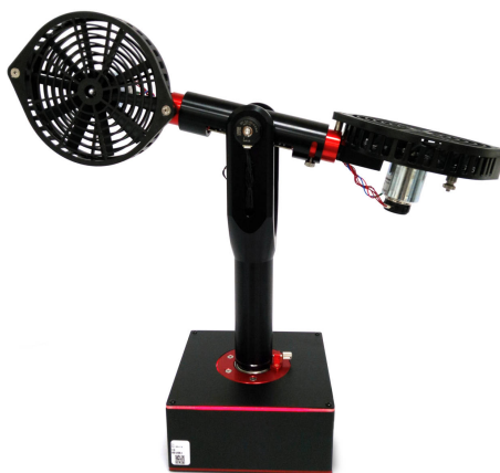
Figure 13. The Quanser Aero 2 testbed in 2-DOF configuration. We turn the fans in the same direction and lock the main arm in order to obtain the 1-DOF configuration of the Aero 2.
