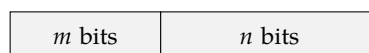
Figure 1.5: A number in Qm.n or UQm.n format is interpreted as an integer scaled by 2^{-n} .
