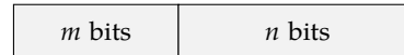
Figure 1.5: A number in Qm.n or UQm.n format is interpreted as an integer scaled by 2^{-n} .
